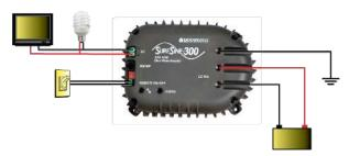
high temperature and low voltage disconnect. Recovery from most faults is automatic
